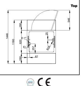
Electric Supply voltage: 220-240 V/1N ph/50/60 Hz Electrical power, max: 0.62 kW **Key Information:** N° of doors: 1 External dimensions, Width: 770 mm External dimensions, Depth: 1180 mm **External dimensions, Height:** 1154 mm Net weight: 82 kg Shipping height: 1184 mm Shipping width: 810 mm Shipping depth: 899 mm Shipping volume: 0.86 m<sup>3</sup> +105 / +115 °C Set temperature: Top temperature: +105 / +115 °C
